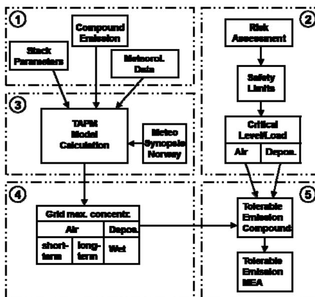
**Figure 1:** Flow scheme of the “worst case” method: 1) Emission input and local meteorological input; 2) determination of critical loads and levels for inhalation exposure, drinking water and aquatic environment; 3) dispersion calculations; 4) maximum air concentration and wet deposition fluxes in the grid obtained from the model run; 5) determination of tolerable emission amounts for the respective compounds and MEA.
