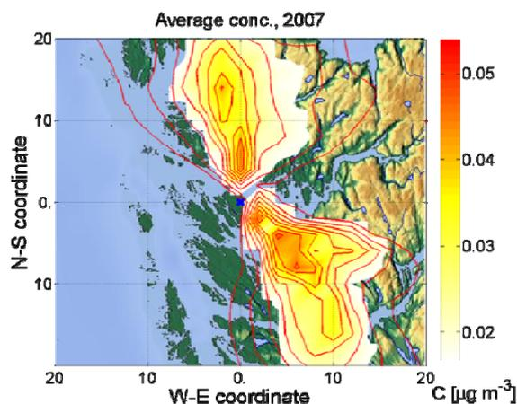
**Figure 2:** Simulated yearly mean MEA concentration in air ( $\mu\text{g}/\text{m}^3$ ) given meteorological conditions of 2007 in the  $40 \times 40 \text{ km}^2$  domain around Mongstad (blue cross).
