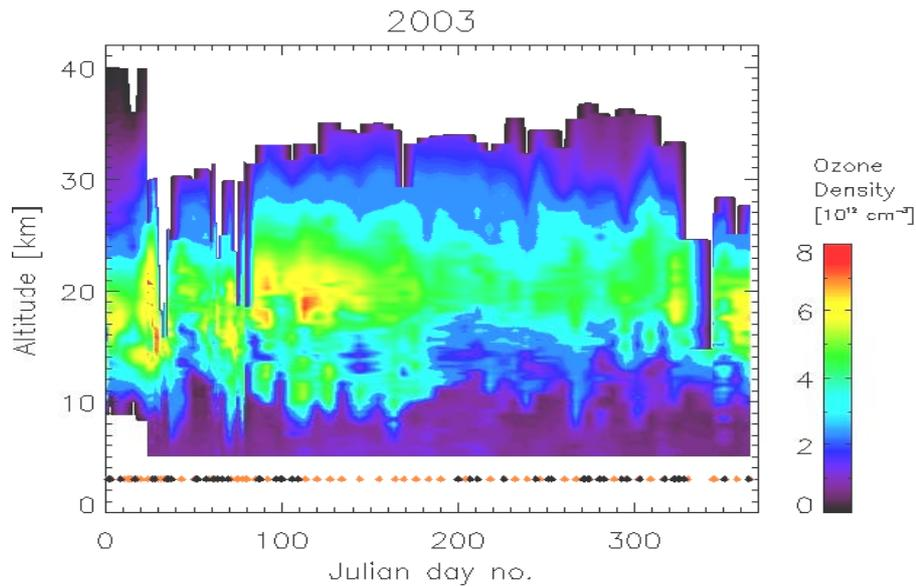
*Figure 5: Ozone profiles measured by the ALOMAR ozone lidar and ozone sondes launched in Sodankylä, Finland, in 2003. The black diamonds at the bottom of the plot mark the times when lidar measurements were performed, while the red diamonds mark days where data from ozone sondes launched from Sodankylä were used. Between the individual measurements the data were linearly interpolated.*
