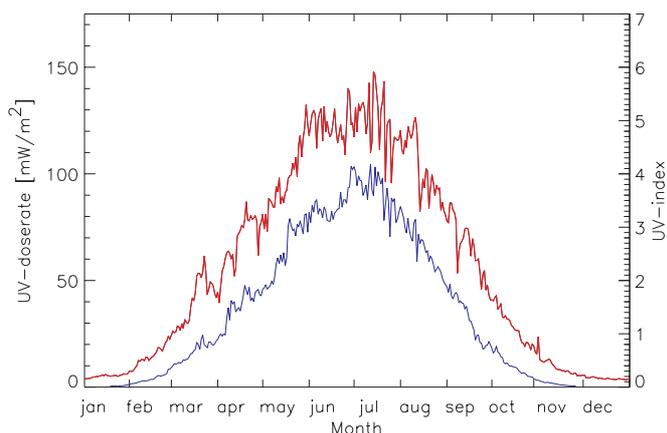
Figure 13: Hourly averaged UV dose rate at noon (between 10:30 and 11:30 GMT) for Oslo and Andøya when the effect of varying cloud cover and ground reflection on the UV dose rate is removed.
