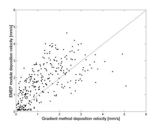
Figure 4: Comparison of modelled and gradient method diurnal average ozone deposition velocities for 2001.
