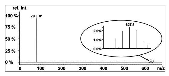
Figure 2: GC/NICI-MS full scan mass spectrum of PBB 153
