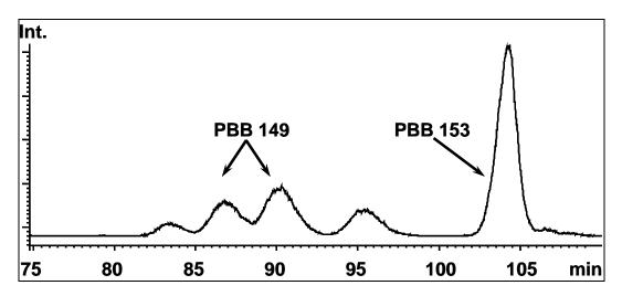
**Figure 3:** GC/NICI-MSMS-single reaction chromatogram (sum of m/z  $625.5 \rightarrow m/z$  79 and m/z  $625.5 \rightarrow m/z$  81) of a purified extract of a bird egg
