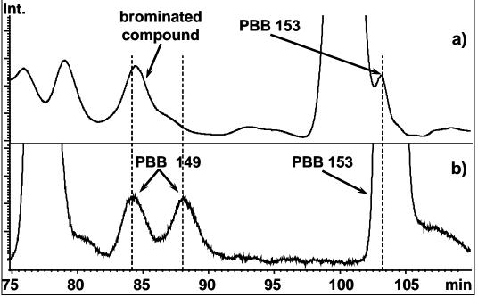
**Figure 1:** GC/NICI-MS-SIM chromatograms (m/z 79 and 81) of (a) the purified extract of a bird egg and (b) the technical product Firemaster BP-6<sup>®</sup>. Dotted lines refer to the retention times of PBB 149 enantiomers and PBB 153
