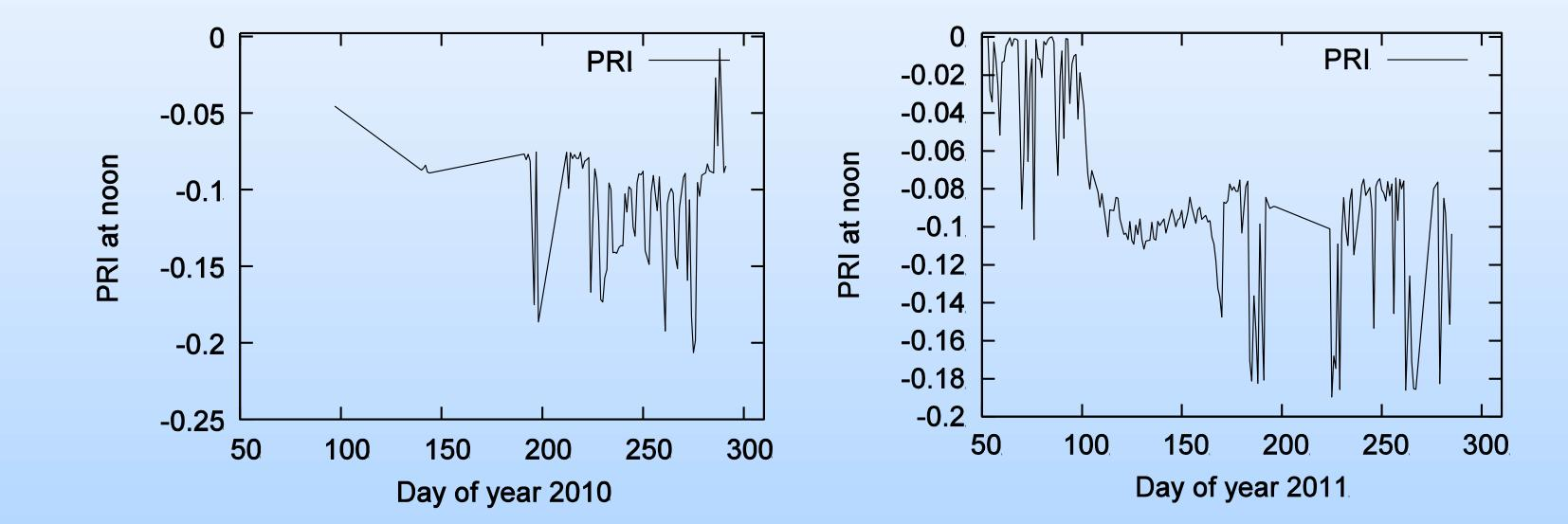
We used two autonomous TriOS Ramses hyper-spectral radiance sensors (radiance and irradiance) in order to measure the spectral radiances during the growing seasons March to end of October 2009-2012. TriOS sensor has a wavelength range of 320 - 950 nm. The radiance sensor measured the surface in an oblique off-nadir angle of 52° and the Field of View is 7°. The irradiance was measured with a hemispheric field of view.
