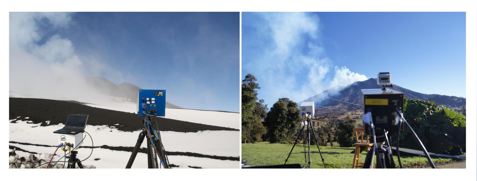
**Fig. 3**: Field measurements using the most recent systems. Left: blue  $SO_2$  camera at a 2850 m plateau at Mt. Etna. Right: golden SO<sub>2</sub> camera monitoring at Turrialba. The white cameras are NILU's IR cameras for volcanic ash and SO<sub>2</sub> monitoring.
