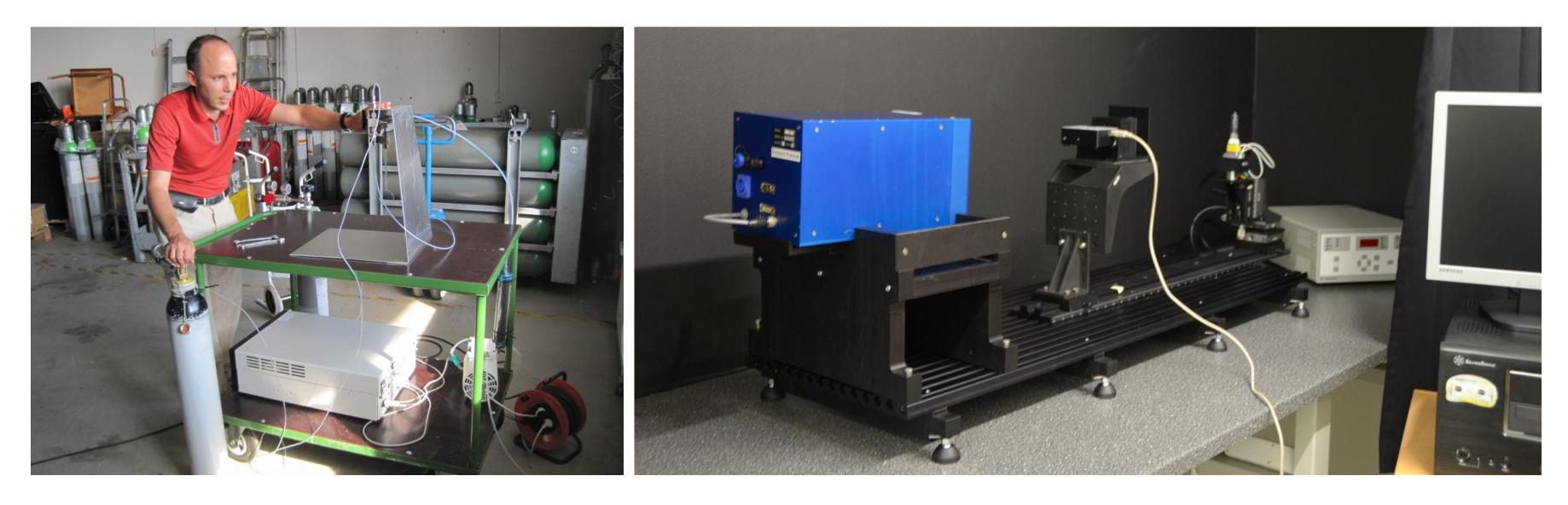
**Fig. 5** : Calibration cell gas filling line (left panel) and laboratory setup for characterization and calibration of the cameras (right panel).
