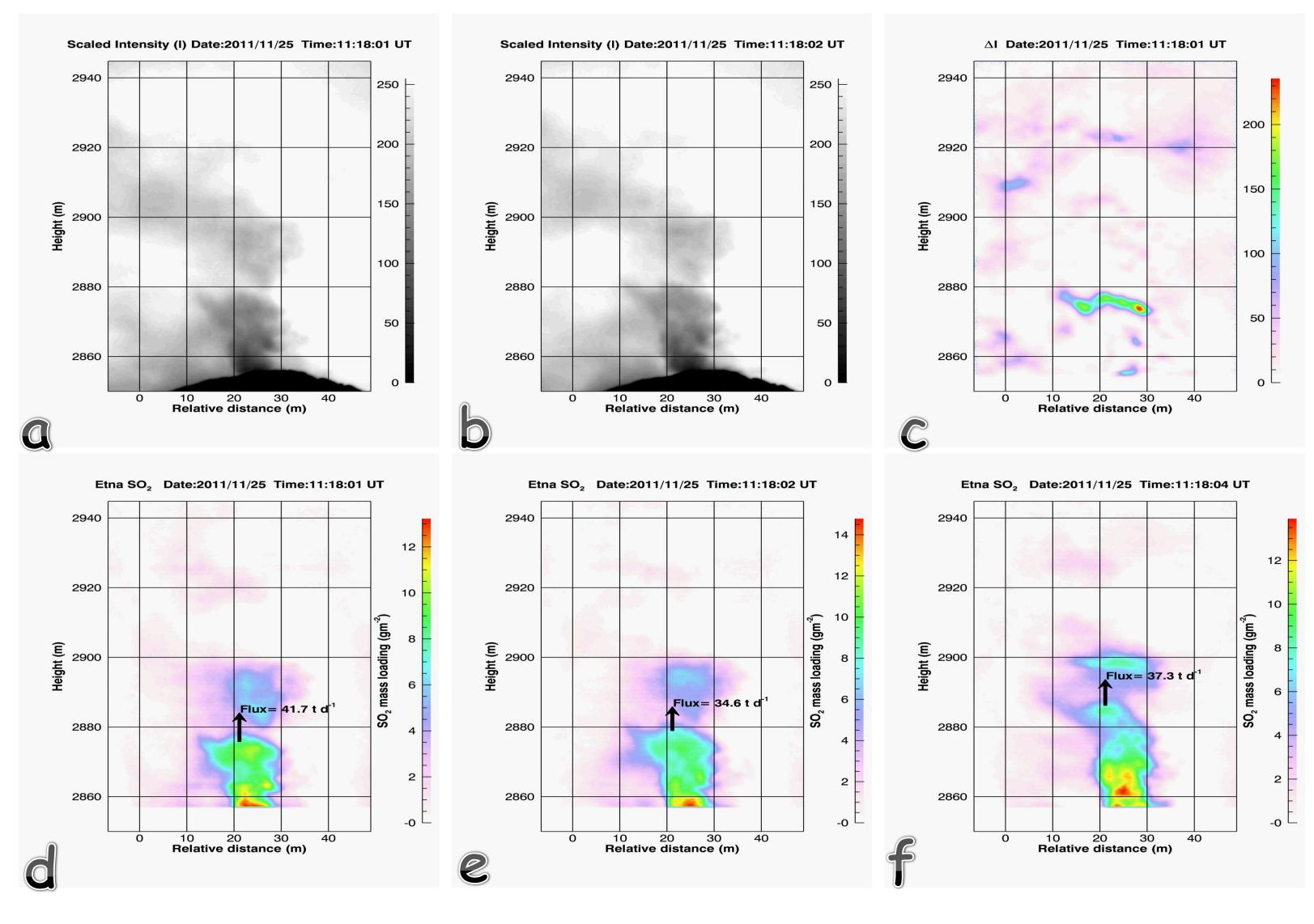
Estimates of SO<sub>2</sub> flux (t day<sup>-1</sup>) were made at a small degassing vent near Torre del Filosofo on Mt Etna, during the recent activity in November 2011. The camera was approximately 1 km from the vent and pointing almost horizontally. Despite intermittent cloud cover the UV camera was able to determine mass loadings and fluxes.
