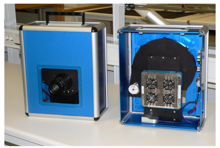
The heart of the second UV camera system (Fig. 2) is a cooled Alta U47 camera, equipped with two on-band (310 and 315 nm) and two off-band (325 and 330 nm) filters.
