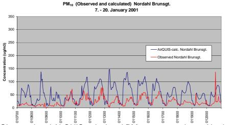
Figure 8: Observed and AirQUIS-calculated PM<sub>10</sub> concentration at Nordahl Brunsgt.
