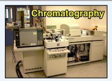
The instrument is a Gas Chromatograph coupled with a High Resolution Mass Spectrometer (GC/HRMS) used for analysis of PBDEs, TBBPA, BPA.
