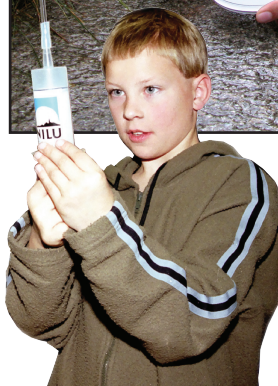
The picture above shows a pupil setting up the sampling equipment for measuring particulate pollution along the school route.
