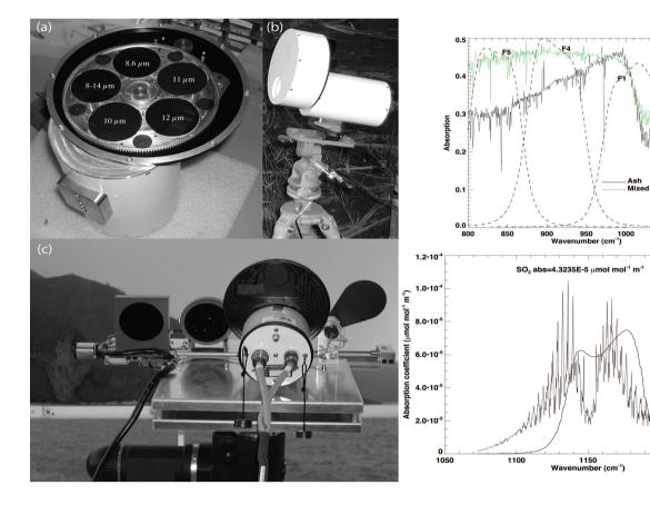
Filters mounted on filter wheel in the arrangement when used for measuring  $SO_2$  gas emissions (central wavelengths in microns are given). (b) "Cyclops" camera mounted on a tripod for field operation. (c) Ship-mounted camera undergoing calibration tests with two moveable blackbodies and an external blackened shutter.
