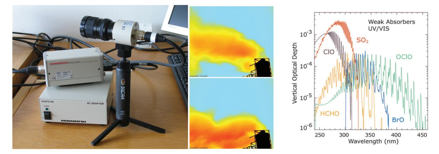
Left: Photograph of the Hamamatsu camera and lens; the basic elements of the NILU UVGasCam. Middle:  $SO_2$  plumes measure by the UVGasCam at an industrial stack. Right: UV spectra of some gases, including  $SO_2$ .
