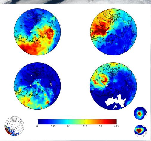
Source sensitivity maps in fraction of the total flow for CO (below) and sulphate (above) for the arctic station Zeppelin, with source regions for "polluted" air to the left and "clean" air to the right.
