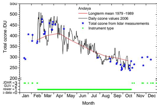
**Figure 2a):** Daily total ozone values measured at ALOMAR, Andøya in 2006 by the Brewer, GUV and LIDAR instruments. The use of the different instruments is shown in the lower part of Figure 2a). The red line shows the long-term monthly mean values from 1979-1989.
