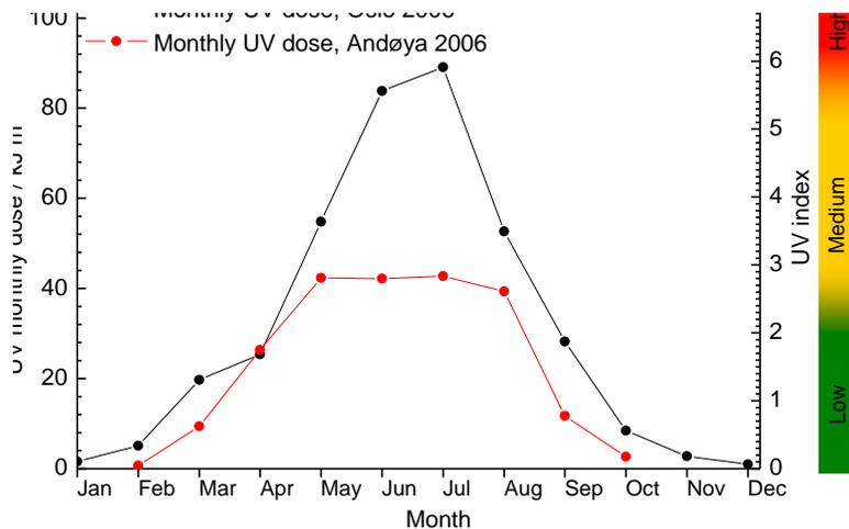
**Figure 12:** Monthly integrated UV doses in 2006 measured with the GUV instruments located in Oslo and Andøya
