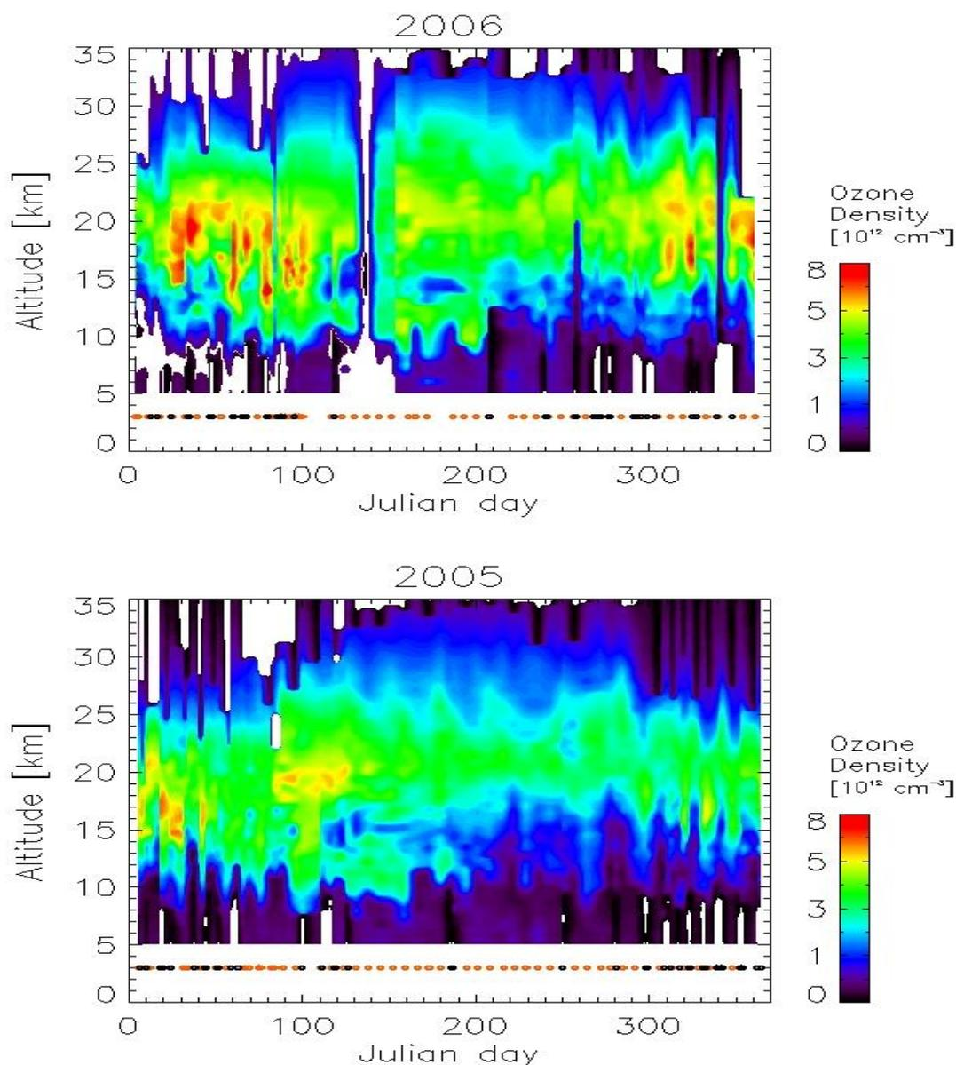
**Figure 4:** Ozone profiles measured by the ALOMAR ozone lidar and ozone sondes launched in Sodankylä, Finland, in 2006 (upper panel) and in 2005 (lower panel). The black dots at the bottom of the plot mark the times when lidar measurements were performed, while the red dots mark days where data from ozone sondes launched from Sodankylä were used. Between the individual measurements the data were linearly interpolated and smoothed with a one-week median filter.
