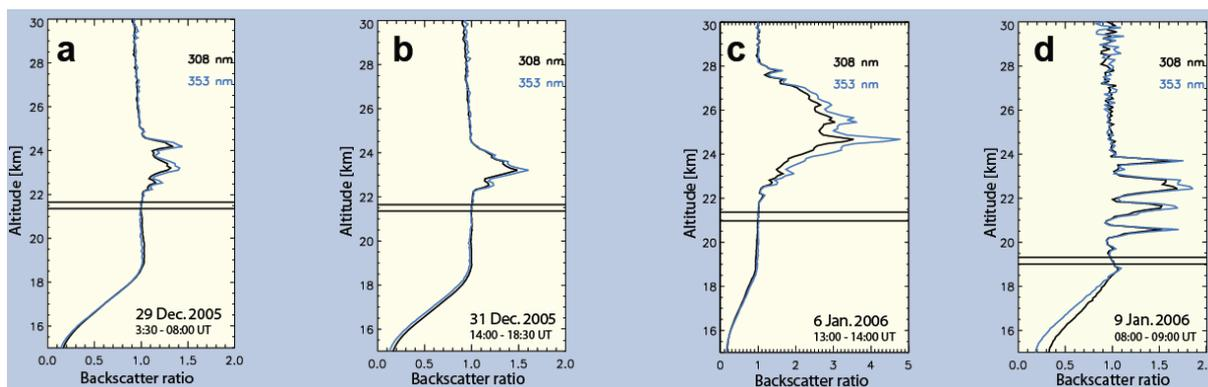
**Figure 3:** Backscatter ratios at 308 nm (black) and 353 nm (blue) as measured by the ALOMAR ozone lidar. From left to right: Observations made on 29 December, 31 December, 6 January and 9 January. Note that the scale of the abscissa is different for the 6 January panel, due to the much higher backscatter ratio on that day.
