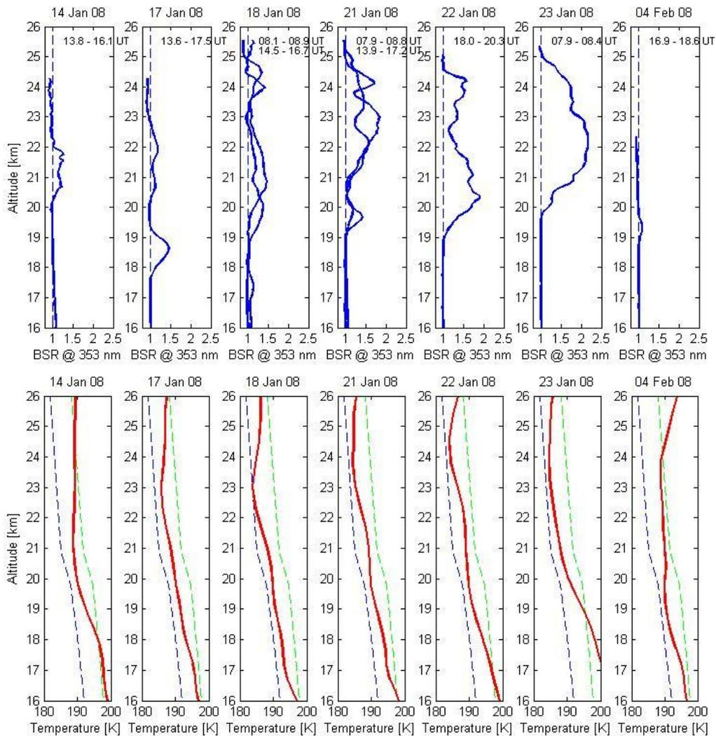
**Figure 12:** Polar stratospheric cloud observations (upper panel) and temperatures (data from ECMWF, lower panel) during spring 2008. The threshold temperatures for PSC type I (NAT) and II (ice) formation are indicated in green and blue, respectively.
