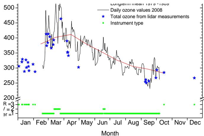
**Figure 2a):** Daily total ozone values measured at ALOMAR, Andøya, in 2008 by the Brewer, GUV and LIDAR instruments. The use of the different instruments is shown in the lower part of Figure 2a). The red line shows the long-term monthly mean values from 1979-1989.
