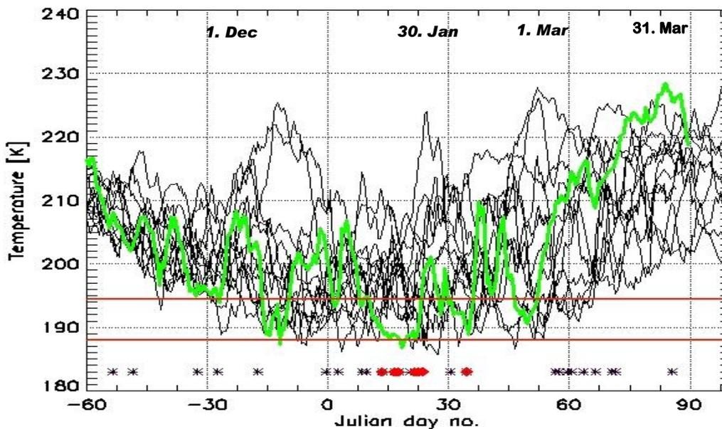
**Figure 11:** Stratospheric temperatures at ca. 20 km altitude above Andøya 1995/96 and 2007/08 (data from ECMWF). The temperature development during winter 2007/08 is highlighted in green. The two vertical red lines indicate the temperature thresholds needed for PSC type I (NAT) and II (ice) formation. Lidar observations made are marked with \*, PSCs observed are indicated by red symbols.
