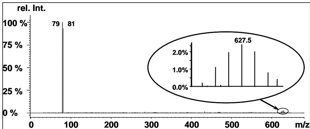
**Figure 2:** GC/NICI-MS full scan mass spectrum of PBB 153
