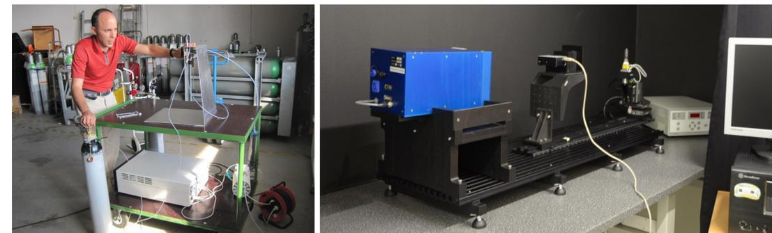
**Fig. 5:** Calibration cell gas filling line (left panel) and laboratory setup for characterization and calibration of the cameras (right panel).
