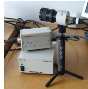
**Fig. 1:** Initial SO<sub>2</sub> camera
