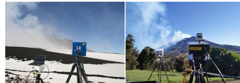
**Fig. 3:** Field measurements using the most recent systems. Left: blue SO<sub>2</sub> camera at a 2850 m plateau at Mt. Etna. Right: golden SO<sub>2</sub> camera monitoring at Turrialba. The white cameras are NILU's IR cameras for volcanic ash and SO<sub>2</sub> monitoring.
